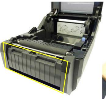
The **Optional Device Compartment** is designed for installation of optional accessories such as the cutter or dispenser unit.
